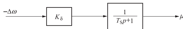
Fig. 7.3 Simplified block diagram of steam turbine governor. T_S —time constant of servomotor; K_δ —amplification factor of speed measuring parts; \Delta\omega —frequency deviation.
