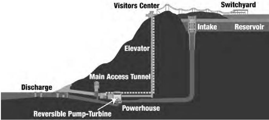
Figure 2-19. Pumped storage power plant.
