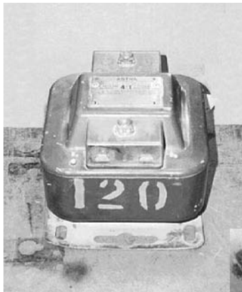
Figure 4-13. Low-voltage PT. Courtesy Alliant Energy.
