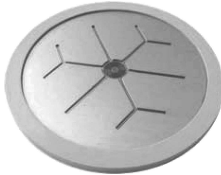
FIGURE 1.6 Top view on a light-triggered thyristor, the line pattern in the blank covering the main cathode area represents the shape of the distributed outermost AG.
