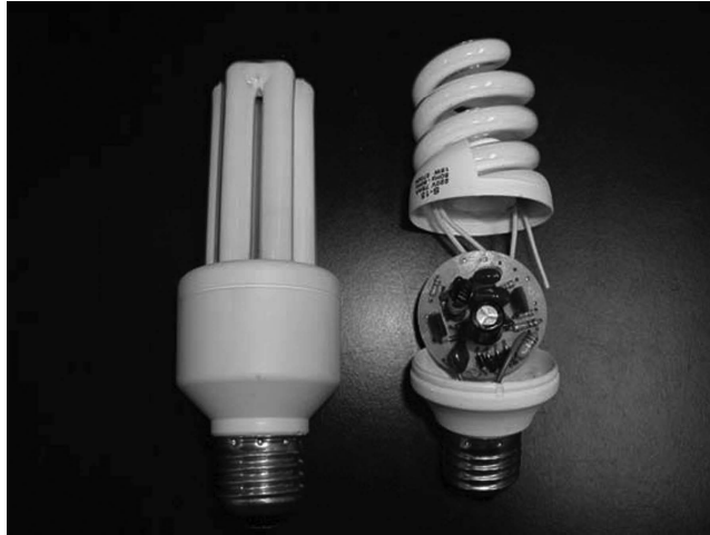
FIGURE 28.2 Photograph of CFL with electronic ballasts and mercury-based fluorescent lamps.
