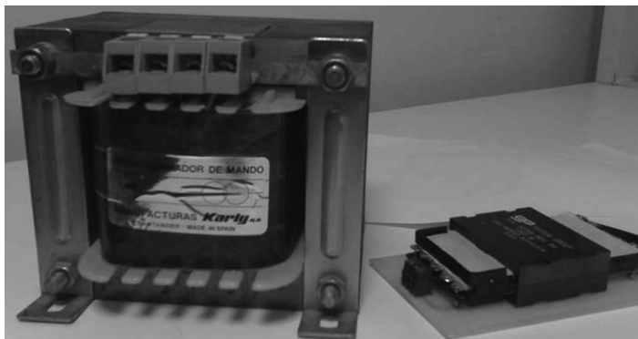
FIGURE 17.15 1 kVA, 50 Hz (left) vs. 1.3 kVA, 125 kHz planar transformer (right).
