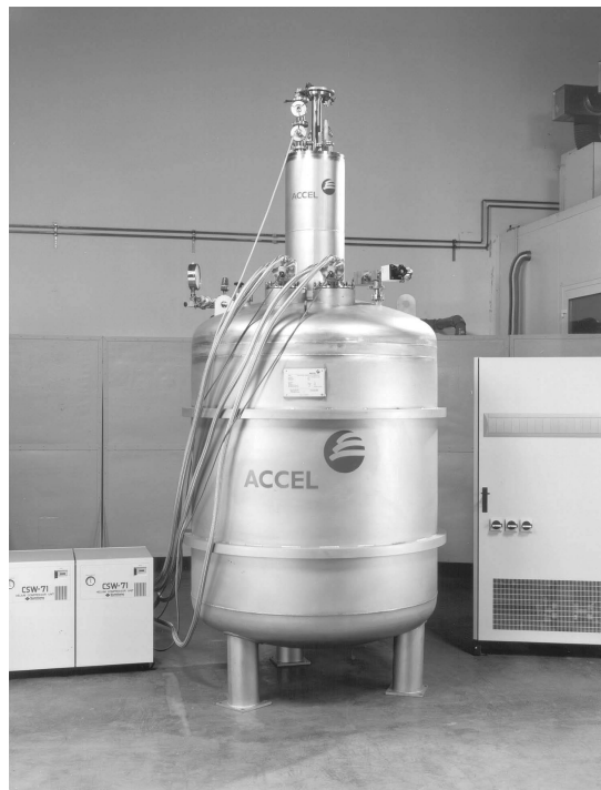
FIGURE 18.6 SMES with 0.6 kWh capacity from Accel. (Courtesy of ACCEL Instruments GmbH.)
