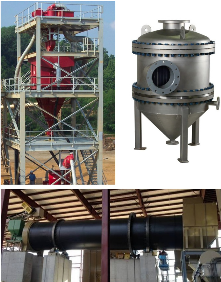
Fig. 14.6 McLanahan Hydrosizer ( upper left ), SWECO hydrocyclone ( upper right ), and Louisville Dryer Corp. rotary gas unit ( lower ).
