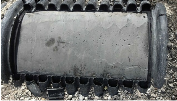
Fig. 6.1 Grout containing FGD gypsum placed at field trial.
