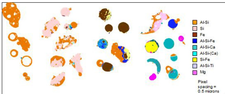
Fig. 2.5 Fly ash particles analyzed by QemSCAN showing the distribution of inorganic phases (minerals and glassy components), defined by different elemental compositions within the individual particles.
