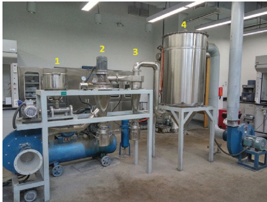
Fig. 10.8 Centrifugal force-based air classifier.
