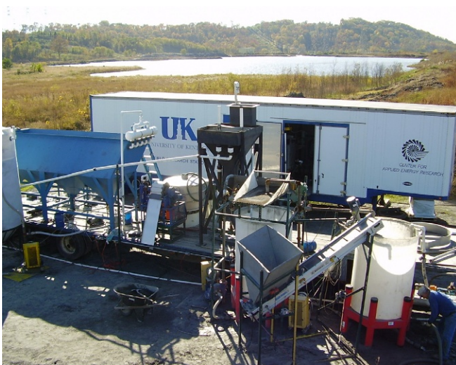
Fig. 14.4 Field demonstration circuitry for recovery of ash from a pond in Northern Kentucky. Flotation cells were housed in the trailer.
