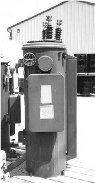
Figure 4-17. Single-phase regulator. Courtesy Alliant Energy.
