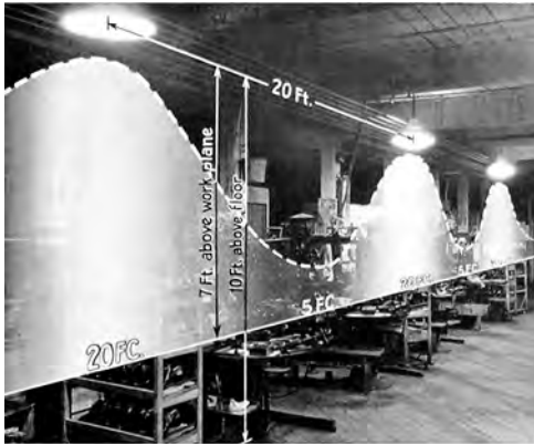
Too wide spacing results in poor distribution, as shown by the top illustration. For best seeing conditions, the illumination throughout the work area should be reasonably uniform. By properly spacing the outlets, as illustrated below, uniformity results.
