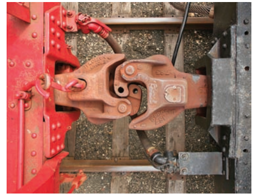
Photo 11.1 The railroad coupler is made of a ductile steel that has a large modulus of toughness.
