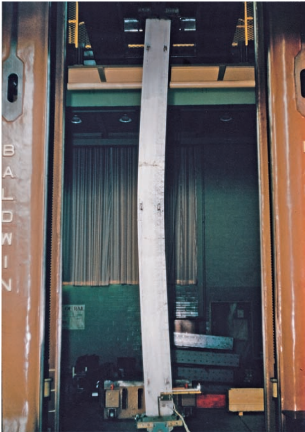
Photo 10.1 Laboratory test showing a buckled column.
