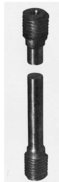
Photo 2.5 Tested specimen of a brittle material.
