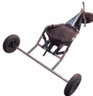
Photo 4.1 For the sport buggy shown, the center portion of the rear axle is in pure bending.
