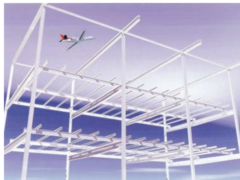
Photo 9.4 The deflections of the beams supporting the floors of a building should be taken into account in the design process.
