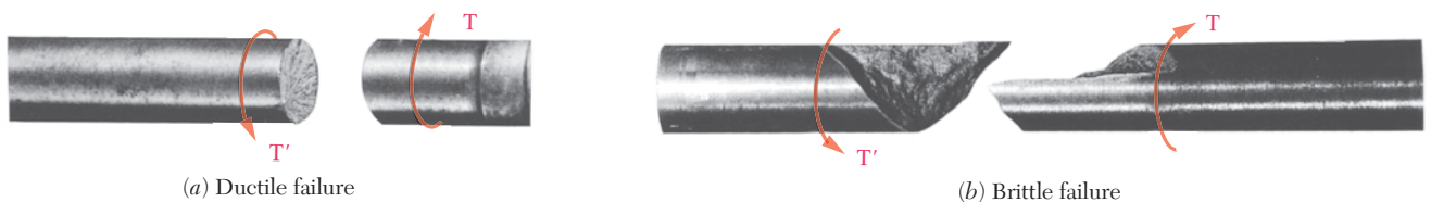
Photo 3.2 Shear failure of shaft subject to torque.
