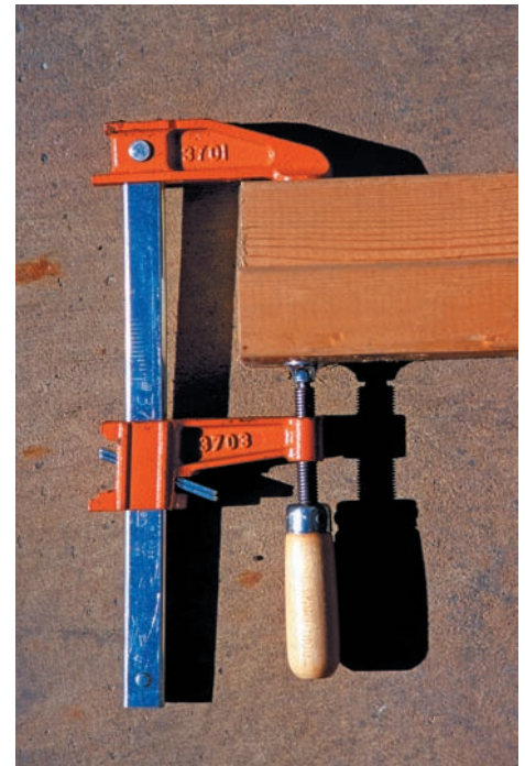
Photo 4.2 Clamp used to glue lumber pieces together.
