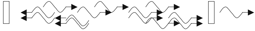
FIGURE 25.22 The mirrored (resonant) cavity of a laser with its front mirror on the right allowing a laser beam to exit. Your imagination is needed to multiply the numbers of photons shown by a tremendous factor of 10^{15} or so.
