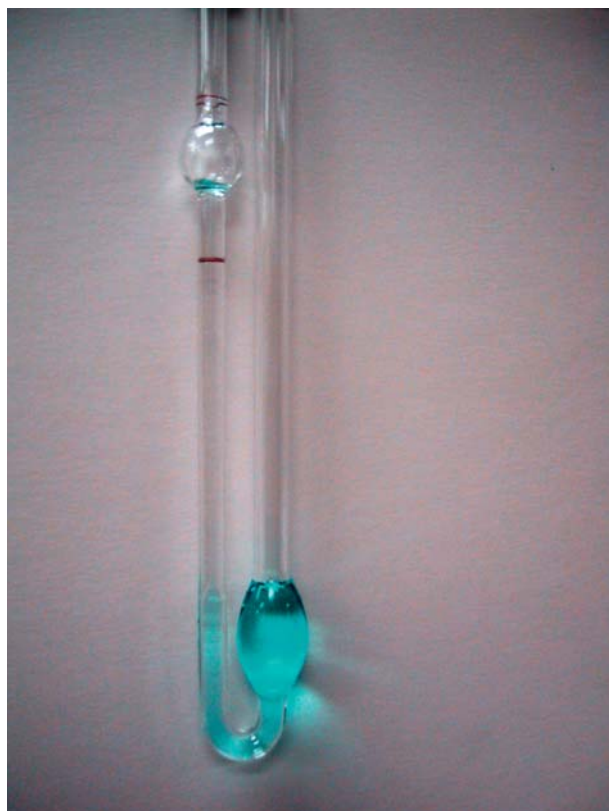
FIGURE 9.4 Capillary viscometer used to measure solvent viscosity by a timing measurement.
