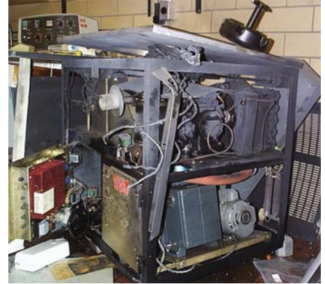
FIGURE 5.27 (upper) Modern ultracentrifuge; (middle) fixed angle rotor; (bottom) centrifuge remains after accident in which a rotor exploded while spinning.
