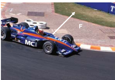
FIGURE 5.21 A car going around a turn has a centripetal force F supplied by the tires.
