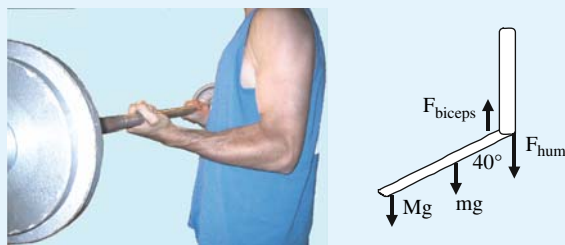
FIGURE 7.16 A person's arm supporting a weight and the force diagram for Example 7.10.
