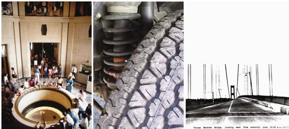
FIGURE 10.1 Oscillating systems: (from left) pendulum at the Griffith Observatory, an automobile coil spring, and the Tacoma Narrows bridge, just before its collapse.
