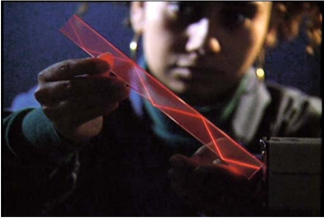
FIGURE 20.20 Total internal reflection in a light pipe.
