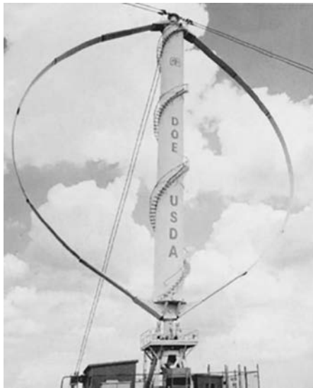
FIGURE 3.2 Vertical-axis 33-m-diameter wind turbine built and tested by DOE/Sandia National Laboratory during 1994 in Bushland, TX.
