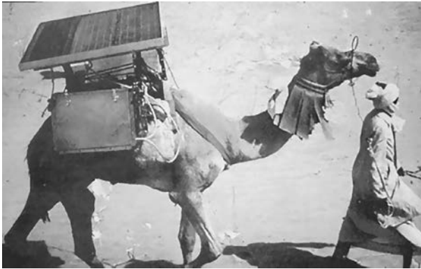
FIGURE 15.2 A traveling clinic uses photovoltaic electricity to keep vaccines refrigerated in the African desert area. (From Siemens Solar Industries. With permission.)
