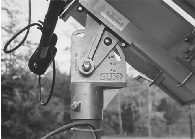
FIGURE 11.19 Actual motor of the sun tracker. (From American Sun Company, Blue Hill, Maine. With permission.)
