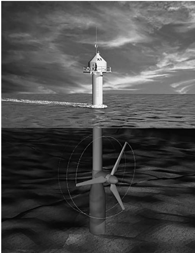
FIGURE 21.3 The 300-kW marine current power generator installed near Devon, U.K. (From Marine Current Turbines Ltd., Bristol, U.K. With permission.)
