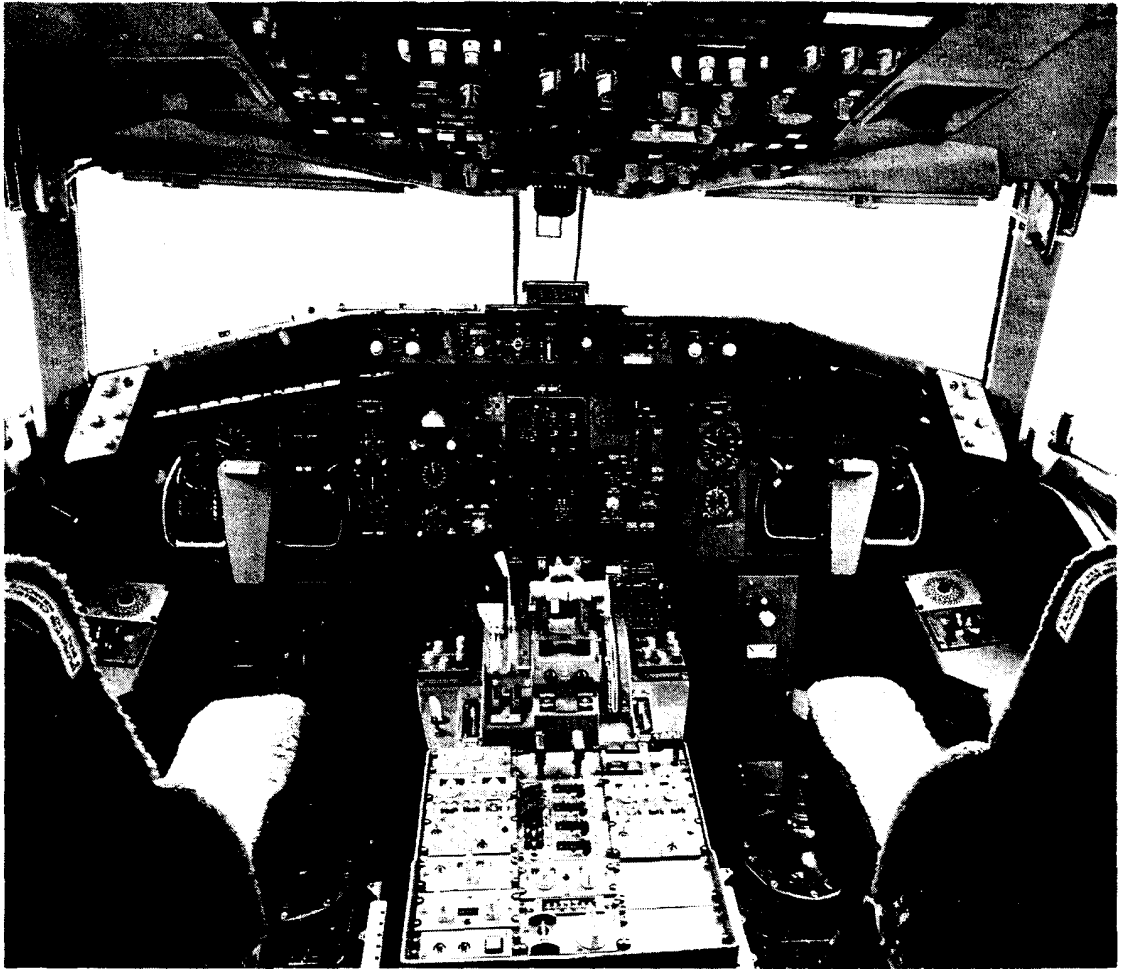
Two-crew-member airline flight deck. The digital electronics include an automatic flight control system (i.e., "automatic pilot"). (Courtesy of Boeing Airplane Company.)
