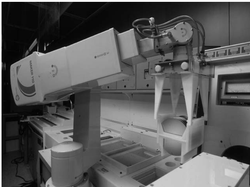
FIGURE 7.9 A robot used in the manufacturing of semiconductor random-access memories (RAMs) similar to those in personal computers. Steady-state error is an important design consideration for assembly-line robots.
