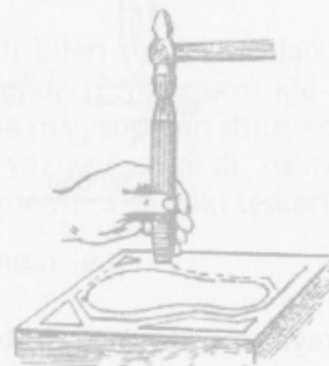
3.8- rasm. List metalldan zagotovka kesib olish.
