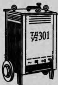
3.3-rasm. Yoy bilan dastaki payvandlash uchun chulg'amlari suriladigan transformator.
