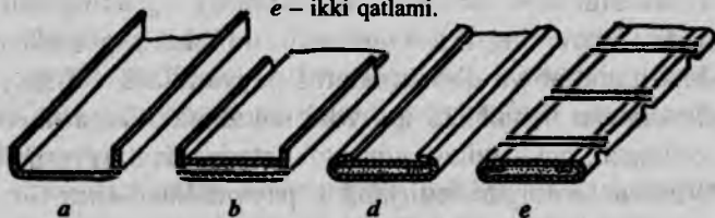
4.5-rasm. Kukunli tasmani tayyorlash sxemasi:
