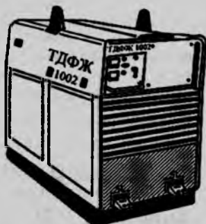
3.4-rasm. Flyus qatlami ostida yoy bilan payvandlash uchun ТДФ transformatori.
