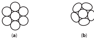
Figure 5.3 Stranded conductors (a) circular type is generally used for 1-phase applications, and (b) compact circular type is used for 3-phase applications.
